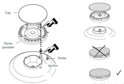
Figure 32 Auxiliary, rapid and semi-rapid burner parts
